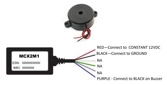
To connect your buzzer, first connect the RED wire from your buzzer to a +12 power source. Next, connect the BLACK wire from the buzzer to the PURPLE wire on your GPS tracker.
